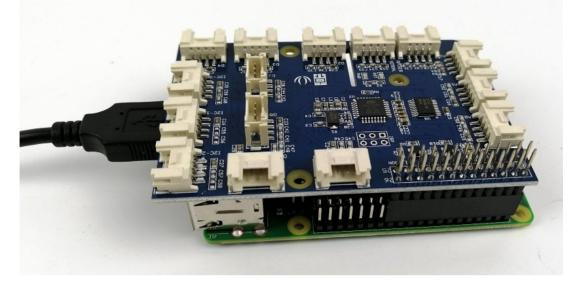
2. Plug the DHT11 Sensor (Blue color) to port D4 on GrovePi.
